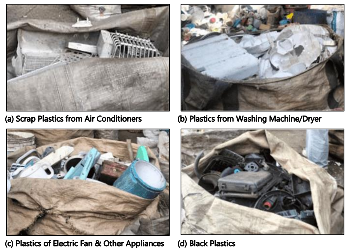
Figure 1. Residual Waste Plastics in Site A
