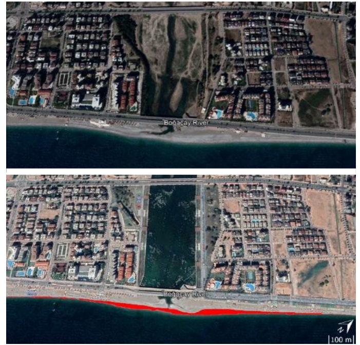
Figure 3. Coastal erosion of the Konyaaltı shoreline between October 2017 (top) and August 2019 (down).
