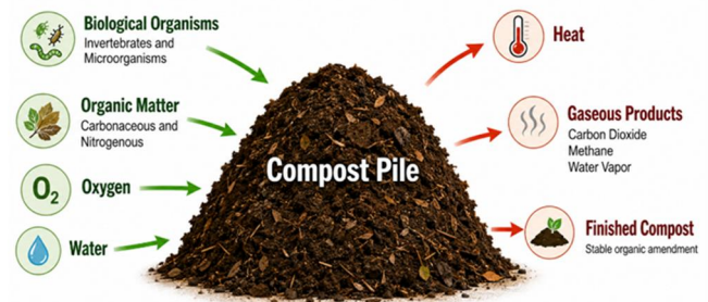
Figure 1. Basic composting process for a static pile (inputs and products of composting).
